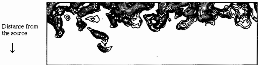
Fig. 9.1. Contours of the kinetic energy on a plane in the flow created by an oscillating grid in a quiescent fluid; the grid is located at the top of the figure. Energetic packets of fluid transfer energy away from the grid region. From Briggs et al. (1996)
